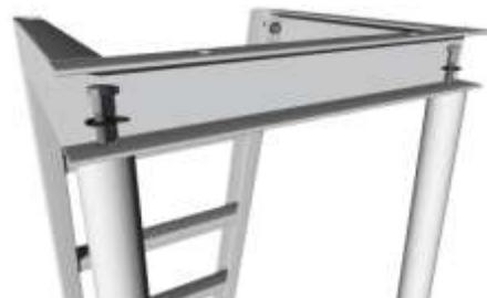
5. **Bolt HANDRAILS** (left and right) to the LADDER assembly with  $\frac{3}{4}$ " bolt/washer, three (3) places each.
