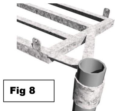
**9. Install the deck frame** onto the centerpost (Fig 8) and support it with a temporary prop.
