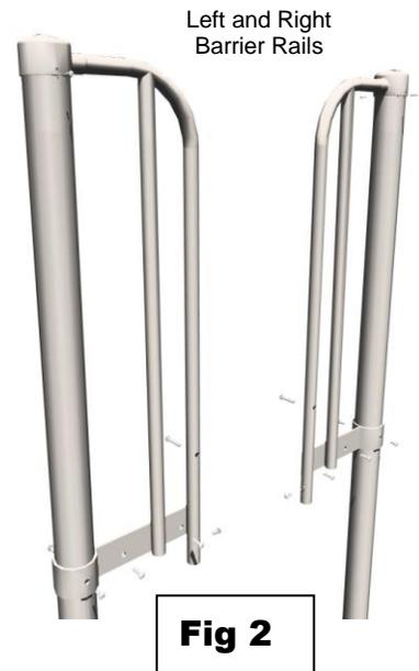
1. a) **Install the metal barrier rails** (Fig 2), one left and one right, onto the ladder posts (Fig 3) making sure that the threaded holes for the plastic siderails face inboard. Use  $\frac{3}{4}$ " bolts through holes in the 4" round socket, into the threaded holes in the post.
