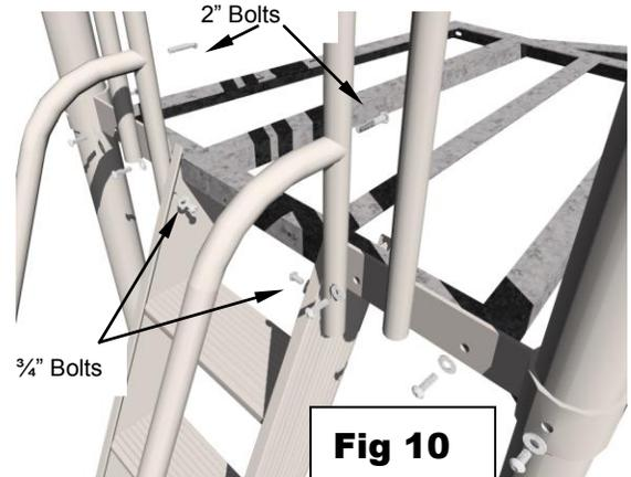
**14. Install the slide Entry section**, plastic Deck Cover, and Strut. Align Deck Cover and Entry vertically using 1/4" bolt through the Strut, the slotted hole in the front member of the deck frame, and into the threaded insert in the plastic Entry module. Attach the lower end of the Strut to the ladder post using #14 U-drives.
