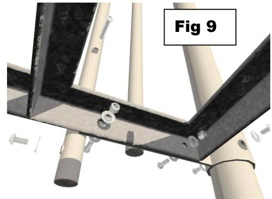
**11. Check all adjustments.** Confirm that the **deck frame is level** and posts are plumb. If necessary, adjust the plastic slide vertically and rotationally by loosening the setscrews in the exit support. The deck frame must be level longitudinally, and posts plumb, to ensure proper fit of all succeeding components.
