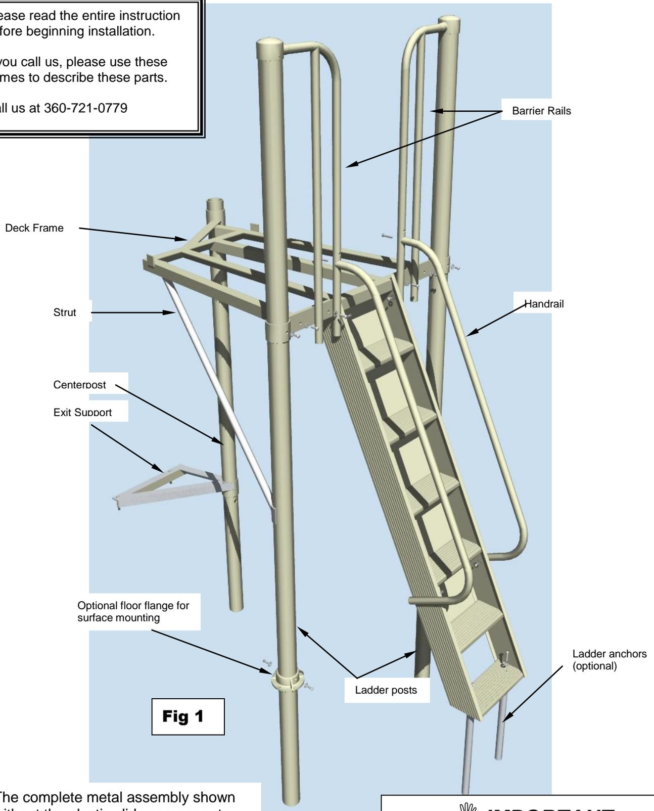
The complete metal assembly shown without the plastic slide components.
